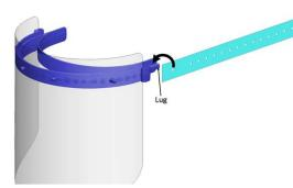
5. Attach the first hole on the adjustable head strap to the protruding lug on one side of the headband.
