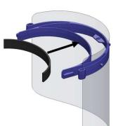
8. If desired, remove adhesive backing and fix foam strip to areas of headband in contact with skin (forehead and side of head) for additional comfort.
