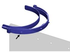
2. From the attached side, push the first hole in the transparent shield over the relevant peg on the headband.
