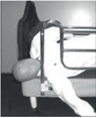
Head & body entrapment because insufficient gap left between head of bed and bedrails.
